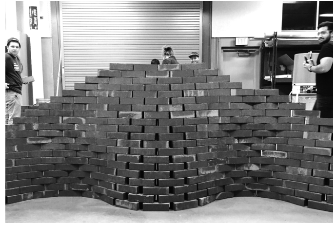
Figure 4: Improvisational Dry Stack Ruled Surface Brick Wall, 4'x12'x4"..
